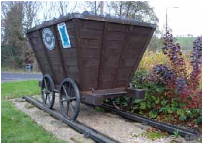
Replica waggon on iron rails and stone sleeper blocks along the waggonway © Jenny Lunn
